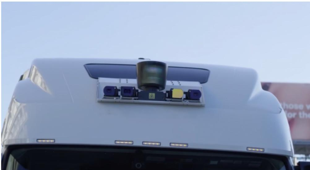
Figura 5.10: Nuevo conjunto de sensores de los camiones de *Uber*.<https://www.constructionequipment.com/video-new-look-and-sensors-uber-self-driving-semi>
