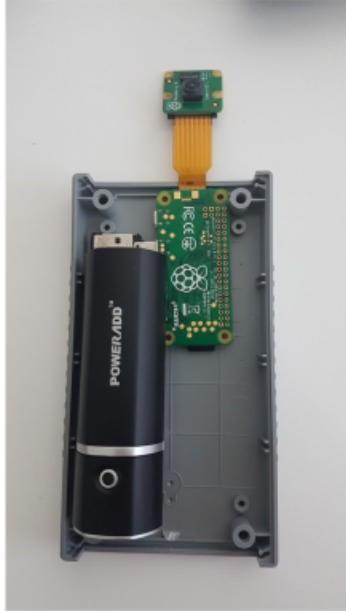
Figure 6.1: Interior of an image capture device
