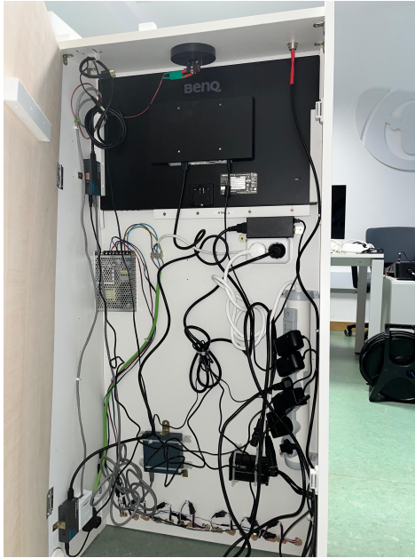
(a) Internal wiring of a lectern, showing power supplies and signal routing.
