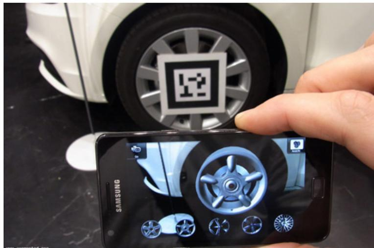
Figure 4.5: Augmented reality marker recognition system
