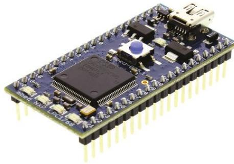
Figura A.3: Microcontrolador mbed. <sup>6</sup>
