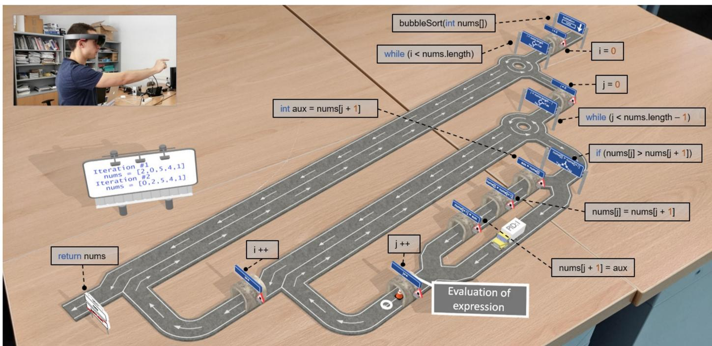
**Figure 4.** Dynamic visualization of the “Bubble sort” algorithm as seen through the AR device. At the bottom right, the execution thread of the program (vehicle) is shown moving towards the breakpoint (traffic cone) and an information panel when the cursor is superimposed on a graphic representation. At the same time, on the left side, a billboard is shown, which prints the status of the algorithm at a particular point of the execution.
