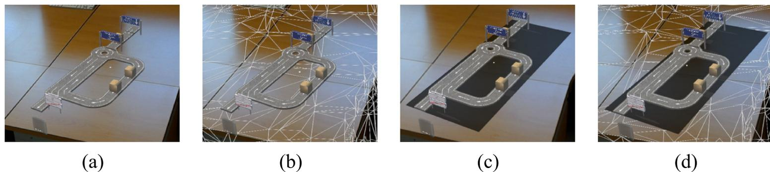
**Fig. 20** Appearance after the execution of voice commands to toggle the visualization of shadows and surfaces; **a** invisible shadows and surfaces, **b** invisible shadows and visible surfaces, **c** visible shadows and invisible surfaces and **d** visible shadows and visible surfaces
