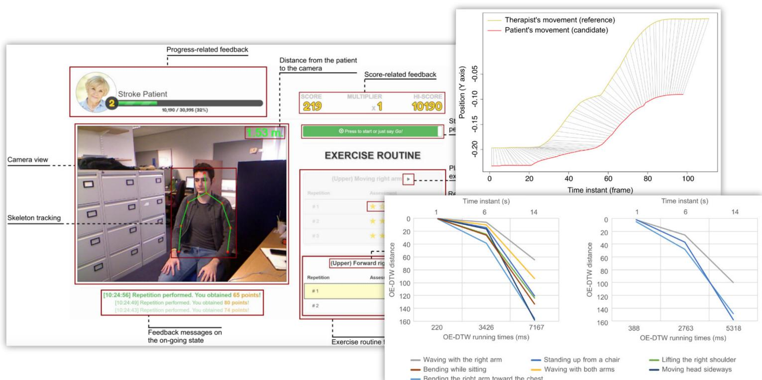
**Figure 2.2:** Main snapshot of the created solution (left) along with a movement curve comparison (top-right) and the recognition of two physical exercises over time (bottom-right).
