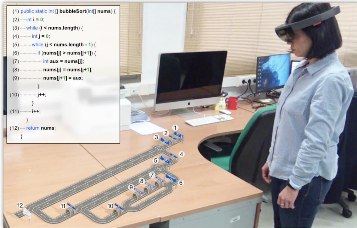
**Figure 2.3:** A photo taken of a user testing the system to visualize programs represented through the ANGELA notation along with the overlaid processed source code relating each graphic representation from the visualization.
