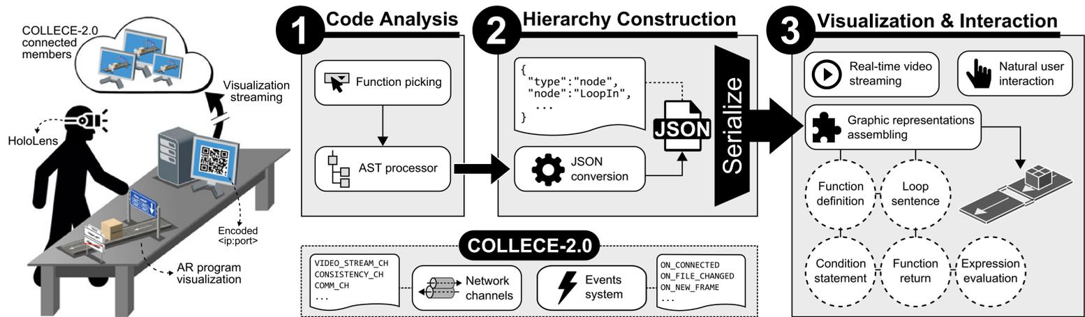
Fig. 14 General overview of the execution flow to generate a visualization from a function selection
