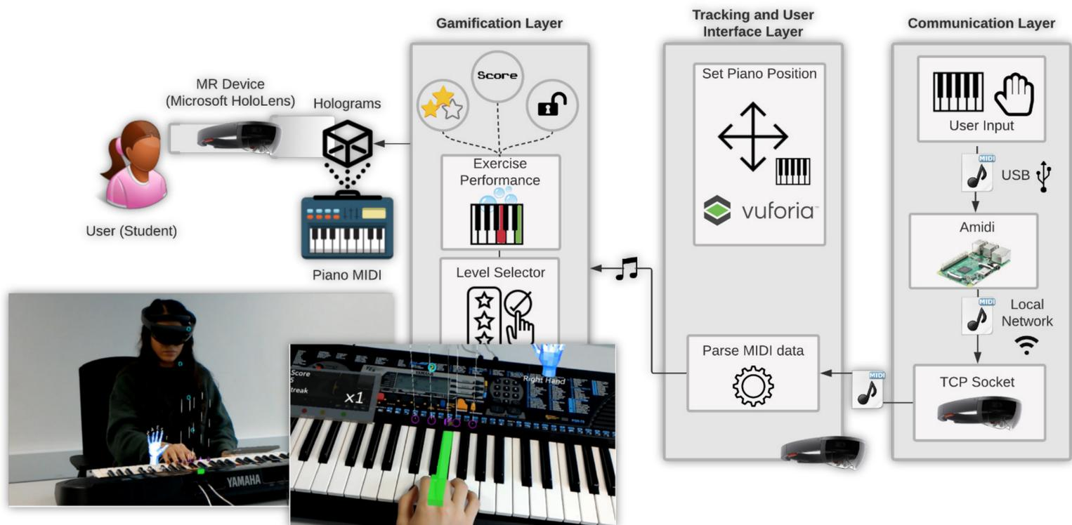
**Figure 2.1:** One of the evaluated user playing HoloMusic XP (bottom-left) and the main workflow diagram of the system (background).
