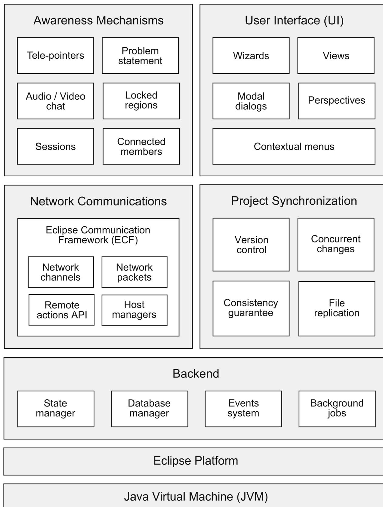
**Fig. 13** Modules of the COLLECE-2.0 platform defining the architecture and the features provided
