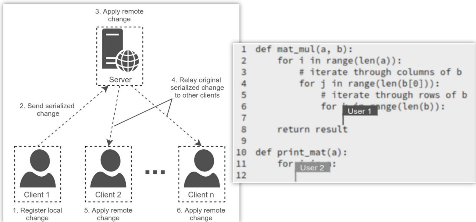
**Figure 2.5:** High level algorithm used to synchronize changes among different users editing the same file (left) and a representation of what would be the future editor of COLLECE-2.0 (right).
